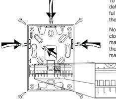
To avoid base plate deformation, be careful when tightening the mounting screws.
