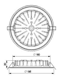
Cut-Out required in ceiling: Ø168mm
