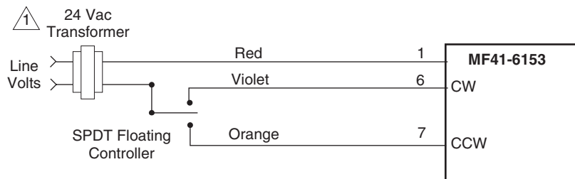
Figure 1 Typical Wiring Diagram for MF41-6153 Floating Actuators.
